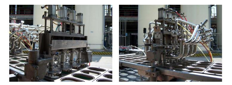
This equipment is fit to the dosing 2 taste or 1 taste\o or decoration of liquid products or half liquid, with valves to single and double entry, opening and closing of the valve commanded by pneumatic pistons, completely adjustable in its position adapts him with any anchorage to all the machine.
