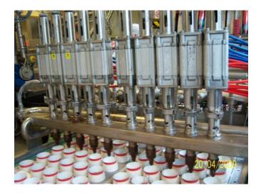
This equipment is fit to the dosing 2 taste or of half liquid products, with valves to double entry, opening and closing of the valve commanded by pneumatic pistons, with flute terminals for a wave dosing.
