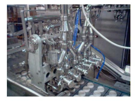
This equipment is fit to the dosing of liquid and creamy products, with valves to single and double entry, opening and closing of the valve commanded by pneumatic pistons, completely adjustable in its position adapts him with any anchorage to all the machine. It has a speed of tested production of 60 shots/1s'
