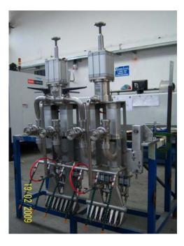
This equipment is fit to the dosing 2 taste or of half liquids products, with valves to double entry, opening and closing of the valve commanded by pneumatic pistons, with flute terminals for a wave dosing.
