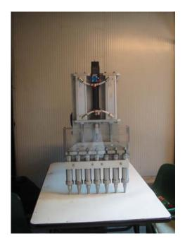
This equipment is fit to the volumetrical dosing monotaste or decoration of liquid products or half liquid, with valves to single entry, opening and closing of the valve commanded by pneumatic pistons, completely registrabile in its position adapts him with any anchorage to all the machine.
