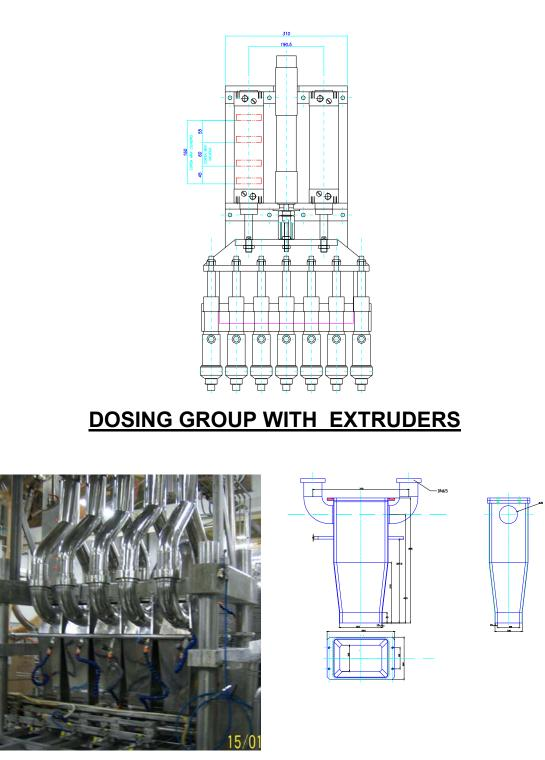
This equipment is fit to the dosing with extruders of creamy products, to double entry, to continuous throw and a group of underlying cut it creates the slice that will be deposed in a tub, completely adjustable in its position adapts him with any anchorage to
