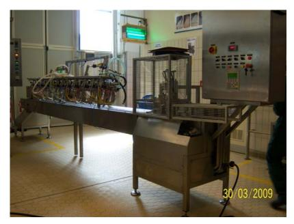
This machine to movement in continuous it is fit to the dosing on little tray of products half liquids and she is essentially constituted by a station of collecting of the tray a series of fillers that they deposit to layers the product and a station of cut and expulsion.
