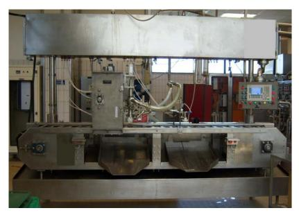
This machine is fit to the dosing of liquid or half liquids products inside a tubs, mini tubs, cups, cones of various kind, on 3 files and she is essentially constituted by a station of collecting of the product, a station of dosing, a station insertion granulates with distributor, a second station of dosing and a station of expulsion of the product.
