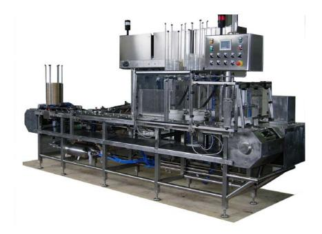
This machine is fit to the wrapping of cakes and she is essentially constituted by a station of collecting of the tray, a station of arrival twisted by side ribbon, a station of assemblage dome and a station of pressing dome.
