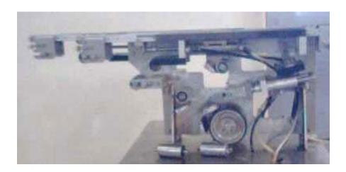
This belt has the possibility to withdraw himself with a command to a pneumatic piston, leaving the belt in movement
