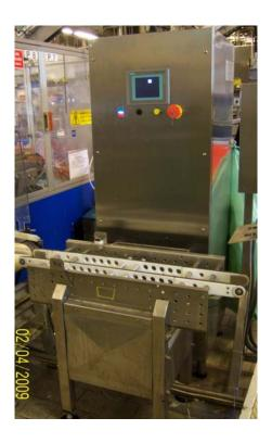
This equipment is fit to weigh a product in movement on a line of production, equipped of cell of load for the weighing, she is managed completely from a control that it allows to plan the weight and the pleasant tolerance.
