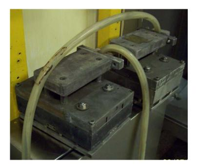
This equipment is fit to the thermo sealing of containers on which it is anticipated film of closing
