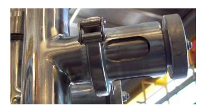
This faucet from 1", 1.5", 2", inserted in a pipeline, throat the passage of the half liquid product
