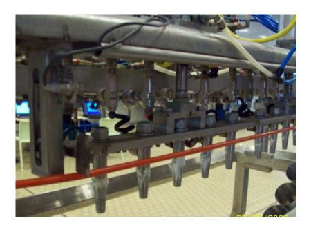
This equipment is fit to practise an imprint in the mixture with aid of sanitary air, that will be filled then by other taste. Completely pneumatic, with a speed of tested production up to 75 shots/1s' with a 99 efficiency%.
